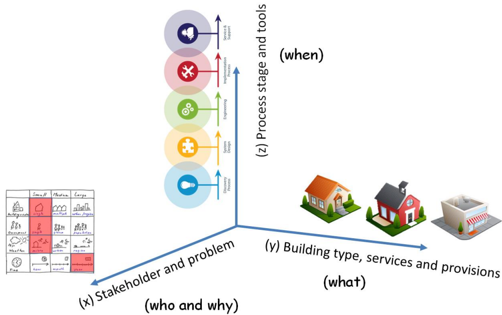
Figure 6: Three dimensions defining main objectives of the energy modelling [Ad van der Aa 2016].
